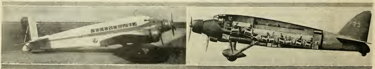
Savoia-Marchetti S-73, a tri-motored passenger plane for 10-18 persons, powered by Gnome & Rhone 9KFR engines of 600 h.p. each
